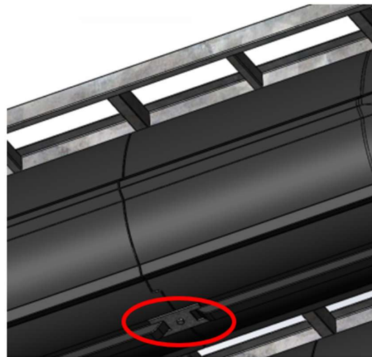
Platform connection with W 1200 S/ W900
